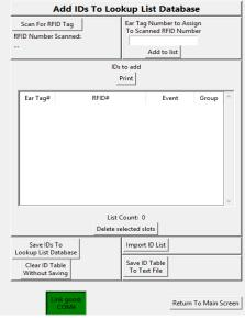
This screen is used to add RFID and visible ear tag numbers to the lookup list database before the list is sent to the *Lightning*ROD reader.
